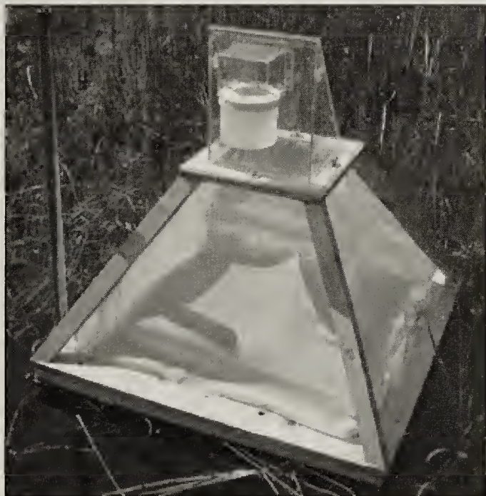
Figure 3: Floating emergence trap used at Site C.
